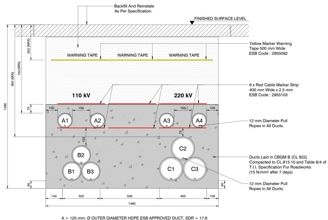
B = 160 mm: Ø OUTER DIAMETER HDPE ESB APPROVED DUCT, SDR = 21
